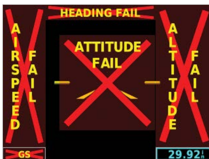
Figure 1-2 G5 PFD Page Failure Annunciations
