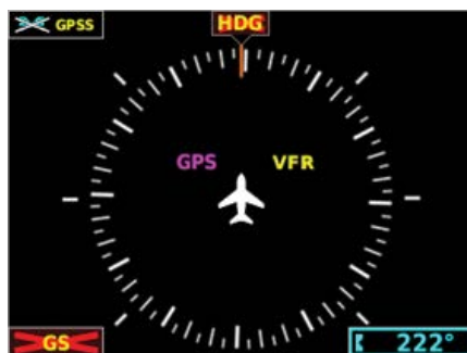
Figure 1-3 G5 HSI Page Failure Annunciations
