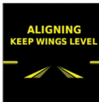
Figure 1-5 Attitude Aligning Keep Wings Level Indication
