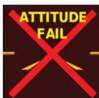
Figure 1-6 Attitude Failure Indication
